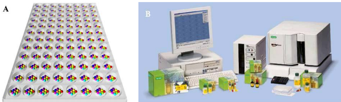
Figure 1: A – Test Plate with Bead Color Sets (multi-colors shown for distinction) B – Luminex® xMAP® 200 Instrument
