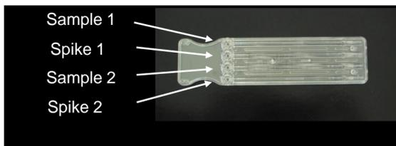
Figure 2: A single use PTS cartridge showing the 4 individual test channels
