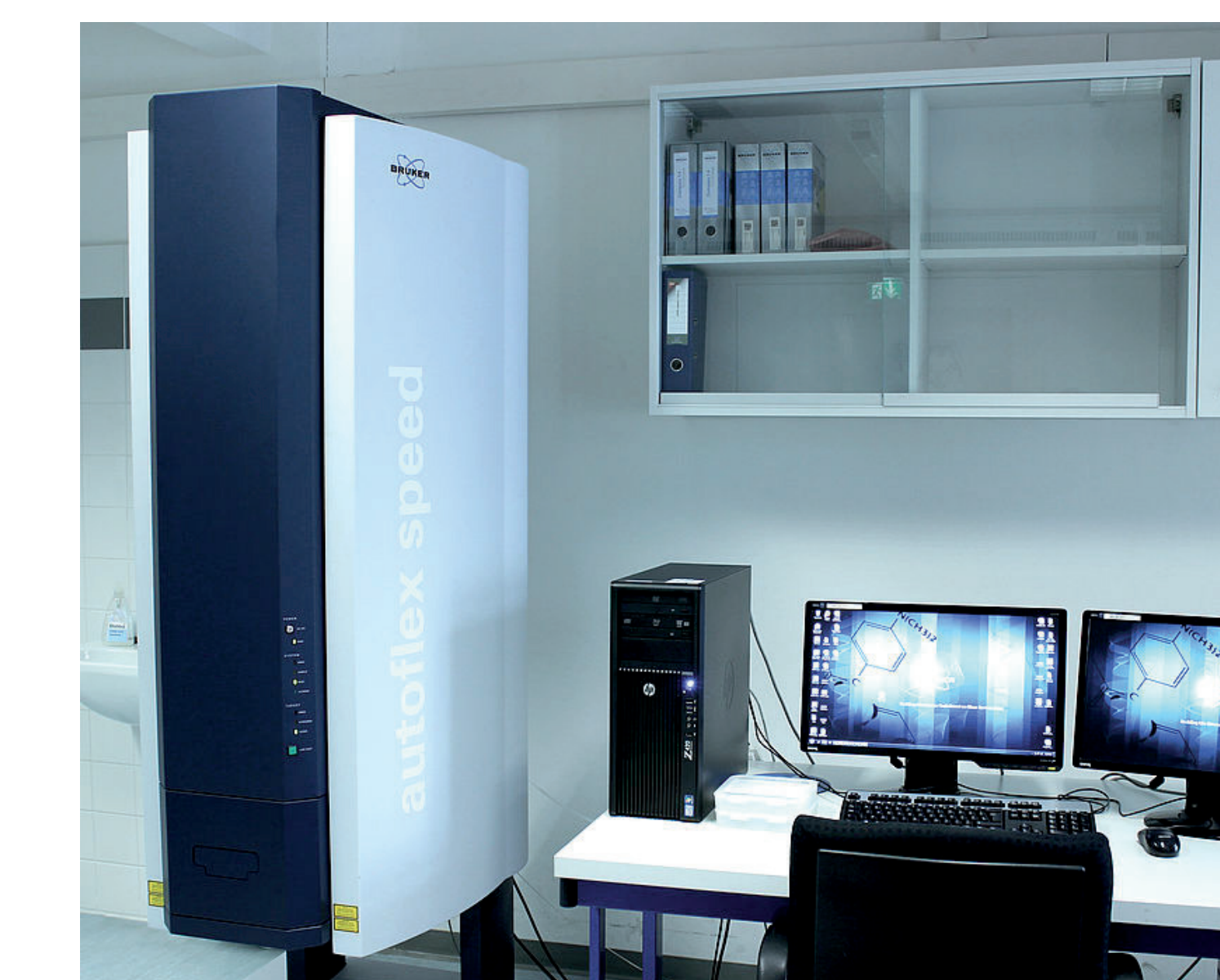
Pictured to the left is the MALDI instrument used in the Charles River laboratories for rapid sample processing that communicates with the Biotracker LIMS application.
