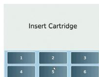
**04** As the reader warms in preparation for use, the **Initializing** message appears. When the unit has reached 37.0 °C, the screen will display the **Insert Cartridge** message.
