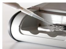
**11** Using a calibrated pipettor, dispense exactly 25 µL of sample into all 4 wells of the cartridge. Be sure to hold the pipette so that the tip is at an angle, and not completely at the bottom of the sample reservoir.\* Click the **Done – Start Test** icon on the home screen to initiate testing.
