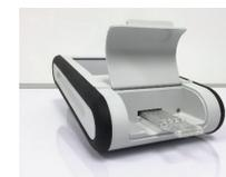
**06** Insert the cartridge firmly into the slot at the front of the reader with sample wells facing up.
