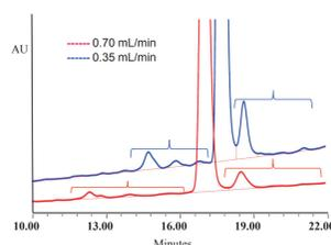
Figure 4. Impact of flow rate on online recovery of related impurities of an oligonucleotide (column: XBridge BEH130 C18, 3.0 x 100 mm, 3.5µm; column temperature: 45°C; counter ion: dodecyltrimethylammonium)
