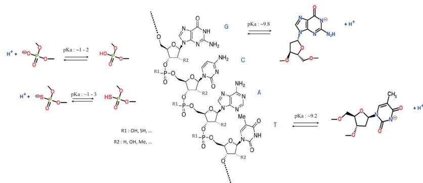
Figure 1. Common acidic dissociations of oligonucleotides in anion-exchange and ion-pairing reverse phase chromatography
