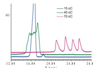
Figure 2A. Influence of column temperature on resolution of oligonucleotides in ion-pairing reverse phase chromatography (column: DNAPac RP, 3.0 x 100 mm, 5µm; counter ion: tetrabutyl- and tetraethyl-ammonium, pH 8.5)
