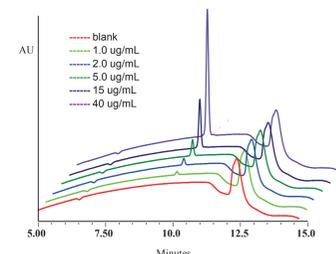
Figure 5B. Chromatography of lipid using UV detection (column: XBridge C18, 3.5 µm, 150x4.6 mm; mobile phase: acetonitrile/isopropanol: ammonium hydroxide, pH 10.5; detection: 204 nm)
