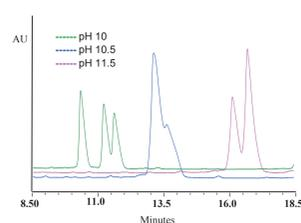
Figure 3. Influence of mobile phase pH on resolution of oligonucleotides in anion-exchange chromatography (column: DNAPAK PA200, 250 x 4.0 mm, 8µ; elution agent: sodium bromide)
