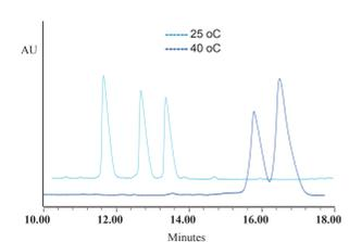
Figure 2B. Influence of column temperature on resolution of oligonucleotides in anion-exchange chromatography (column: DNA PAK PA200, 250 x 4.0 mm, 8µ; elution agent: sodium bromide, pH 11.5)
