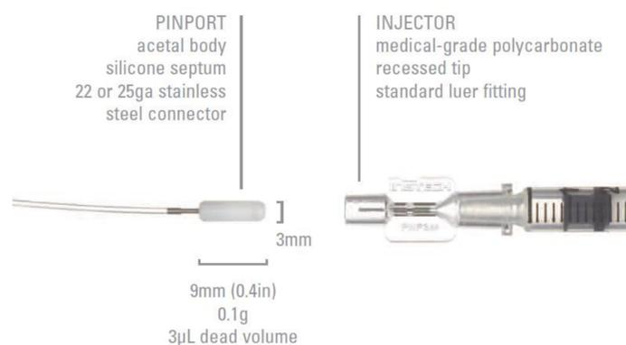
Figure 1: PinPort™ and injector
