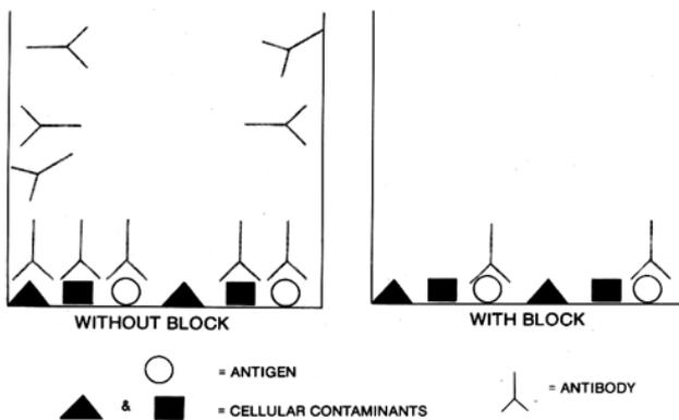
Figure 7. Increasing signal-to-noise ratio: blocking non-specific reactions.
